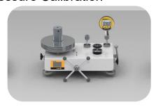
Piston pressure gauge is a standard pressure measuring instrument with high accuracy, high reproducibility and high reliability based on Pascal's law and hydrostatic equilibrium principle. It is a pressure standard with its own pressure source, and the calibration and verification process can be completed by directly installing the instrument under test.
