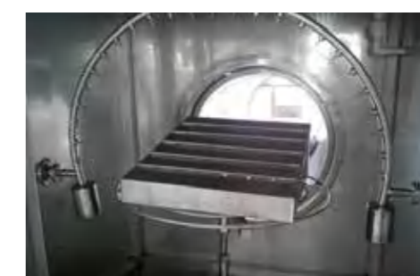
IPX3 IPX4 Rain/Splash Test
